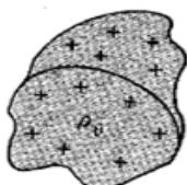
$$dQ = \rho_v dv \rightarrow Q = \int_v \rho_v dv \quad (\text{volume charge})$$
