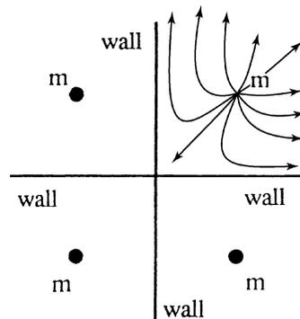
**8.73** Set up an image system to compute the flow of a source at *unequal* distances from *two* walls, as shown in Fig. P8.73. Find the point of maximum velocity on the  $y$ -axis.
